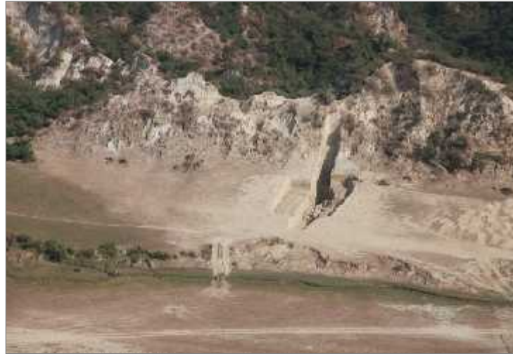
Fig 6.2. Photograph of trench having 70m long, 5m wide, and 8-15m dimension.
