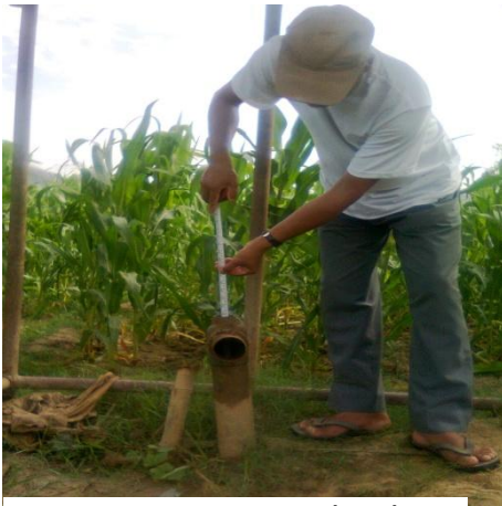
Photo: 2 static water level (SWL) measurements of Shallow tube wells
