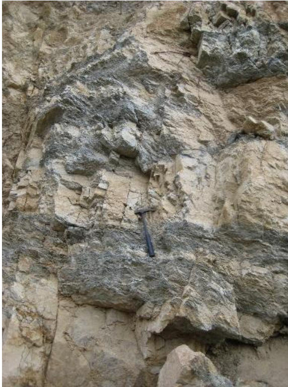
Plate 3.3 Typical interbanding greenish-grey phyllite and greenish-grey dolomite at location OW 25 (picture taken facing north)
