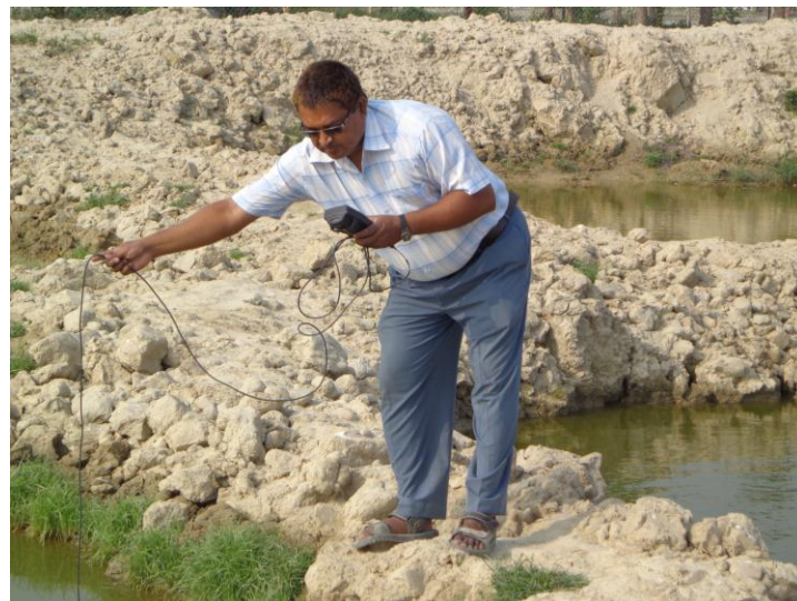
Measurement DO and temp. (DO meter)
