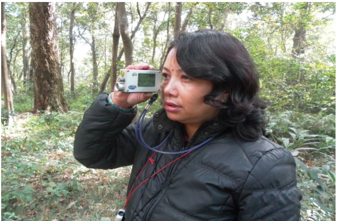
Photoplate 2 – Reading height and distance by Vertex IV
