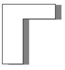
While making the frame of doors and windows, the corner of frame should touch the outer line of *buttom* other wise it is not in perfect shape. Before using *buttom* we measure *tala mathi ko lambai* (length of up and down) with the help of any things like two sticks of equal length, ropes, *bitta*, inch etc.
