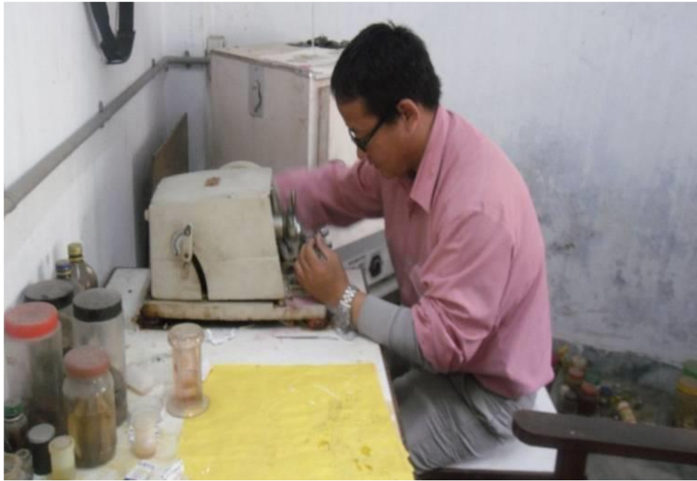
9. Trimming of paraffin embedded blocks with the help of a rotary microtome.
