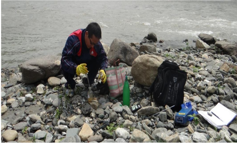
11. Fixation of water sample for estimation of dissolved oxygen (DO) at a sampling site.
