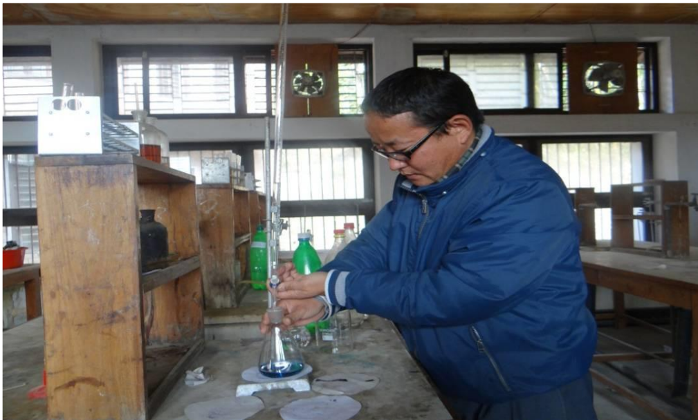
12. Estimation of dissolved oxygen by titration in laboratory.
