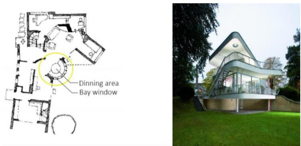
Figure 29: Mohrmann House - Hans Scharoun : An Asymmetric House With A Circular Dining Area (Circular] Plan And View Respt.
