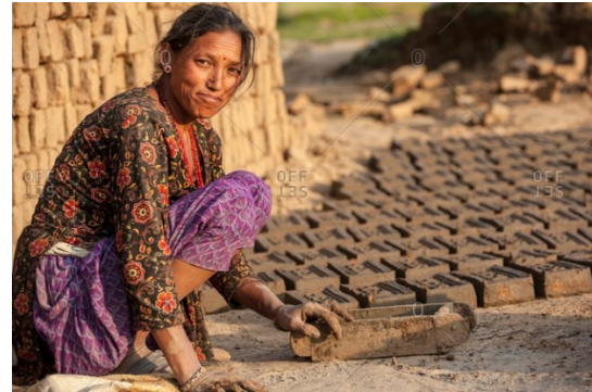
Figure 2.4 Adobe to rebuild the house, Lele village Source:(offset, 2018)
