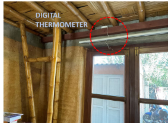
Figure 2: Digital Thermometer placed for thermal measurement
