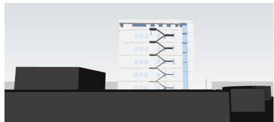
Figure 66: East view with 31% window to wall ratio
