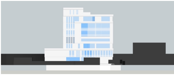
Figure 63: West view with 30% window to wall ratio
