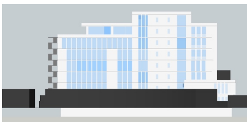
Figure 76: North view with 40% window to wall ratio
