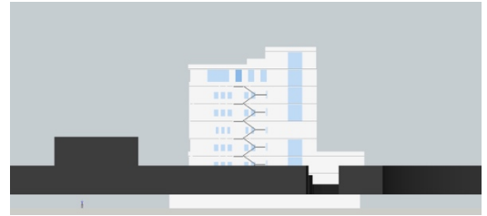
Figure 55: East view with 10% window to wall ratio
