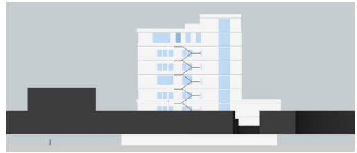
Figure 62: East view with 30% window to wall ratio
