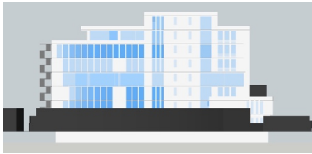
Figure 80: North view with 60% window to wall ratio
