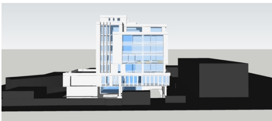
Figure 67: West view with 31% window to wall ratio
