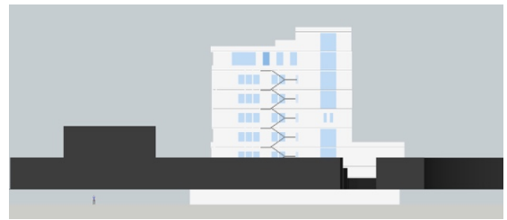
Figure 59: East view with 20% window to wall ratio
