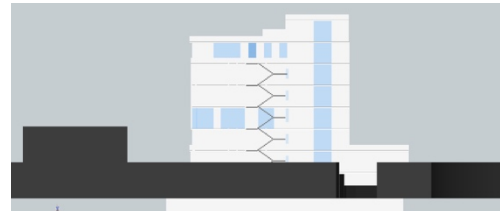
Figure 78: East view with 60% window to wall ratio
