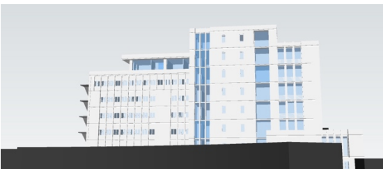
Figure 69: North view with 31% window to wall ratio
