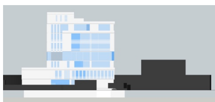
Figure 94: West view with 100% window to wall ratio
