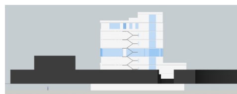
Figure 95: East view with 100% window to wall ratio
