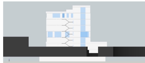
Figure 82: East view with 70% window to wall ratio
