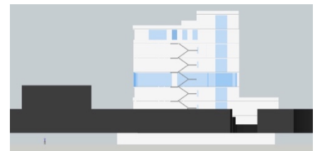
Figure 91: East view with 90% window to wall ratio
