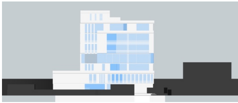
Figure 86: West view with 80% window to wall ratio
