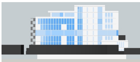
Figure 93: North view with 90% window to wall ratio
