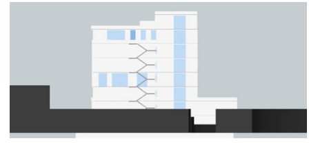
Figure 70: East view with 50% window to wall ratio
