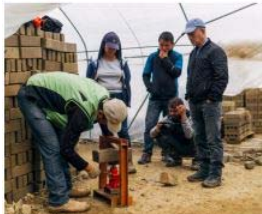
Figure 11 Testing of insite prepared Brick(Devraj & Gustavo, 2021)
