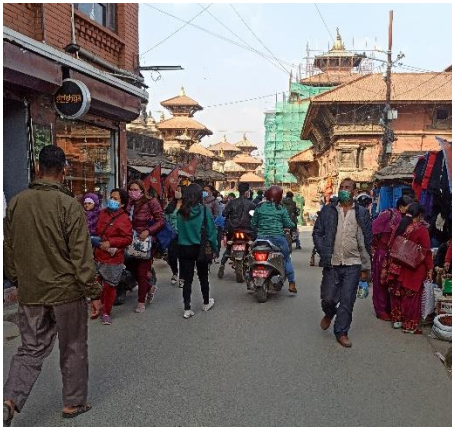
Figure 3-2 Unclear separation between footpath and roadways
