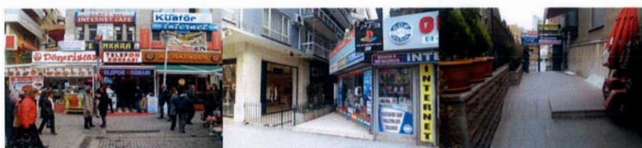
The accessibility of people with disabilities to the building entrances is not available. The main problems in the area are building entrances which are closed by commercial uses, the absence of ramp arrangement or ramps which do not conform to the standards.
