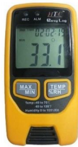
Figure 12: Device used to measure temperature and Humidity
