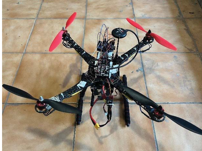
Figure 3.4: Developed UAS (Quad)
