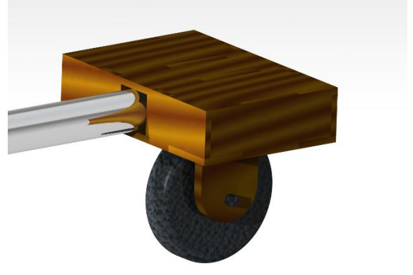
Figure 3. 29: Empennage Connection to Boom
