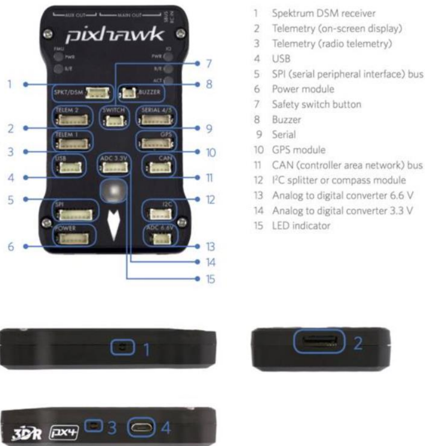
Figure 2. 3: Pixhawk PX4 Flight Controller [18]
