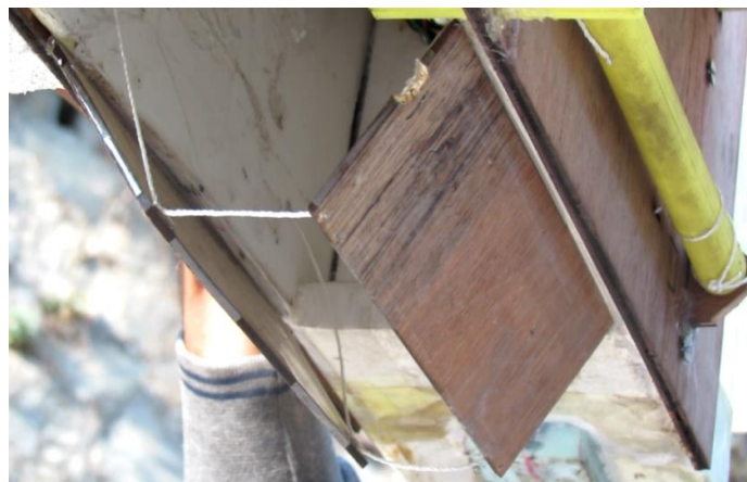
Figure 3. 11: Payload Drop Access Panel
