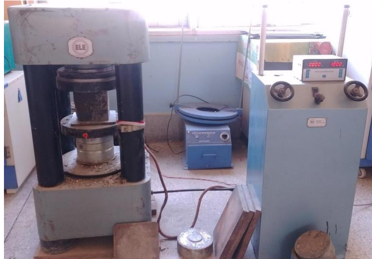
Image 2 Compressive Testing Machine
