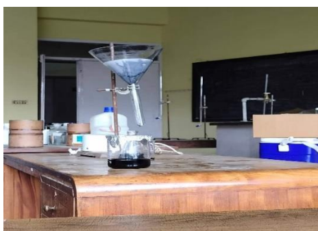
Figure B.8: Washing AC with dil. Water
