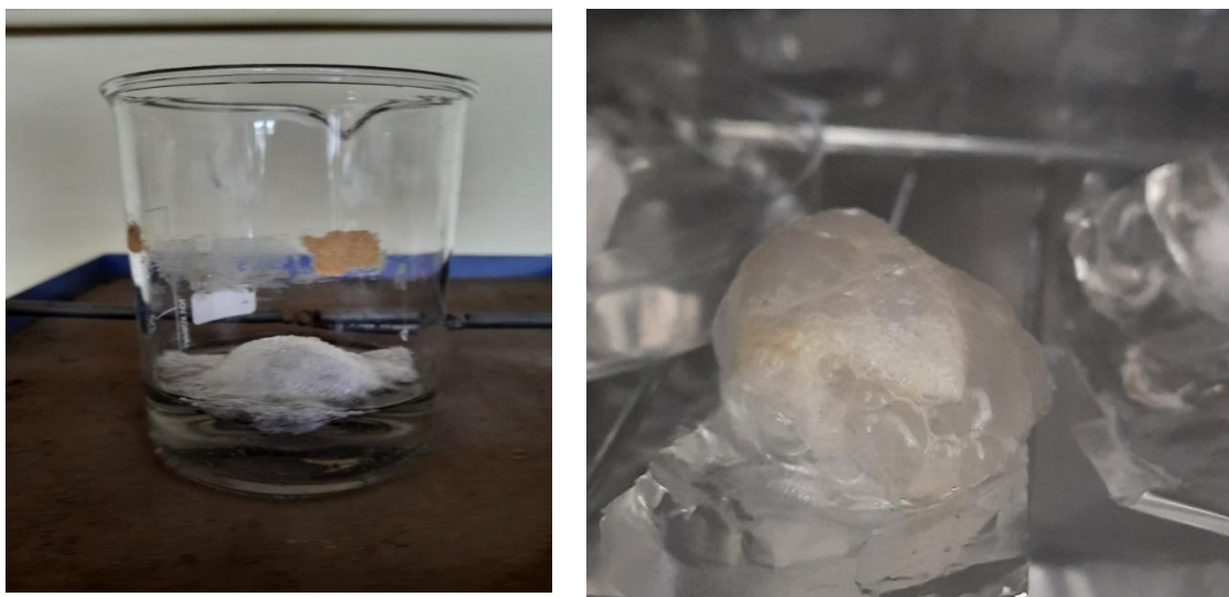
a) PAN fiber in \text{AgNO}_3 and \text{NaBH}_4 solution b) 3D membrane left for washing and drying
