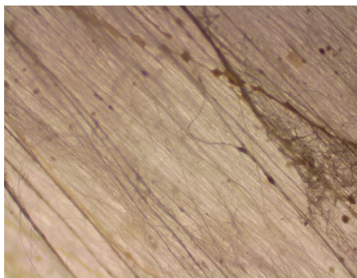
Figure 8 Optical image of pristine PAN fiber under a) 4x and b) 10x zoom
