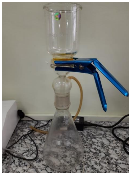
Figure 6 Filtration setup of water and oil sample
