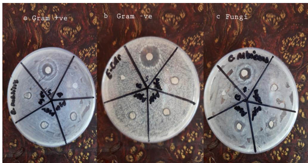
Figure 22 Zone of inhibition test for Ag-Br PAN fiber
