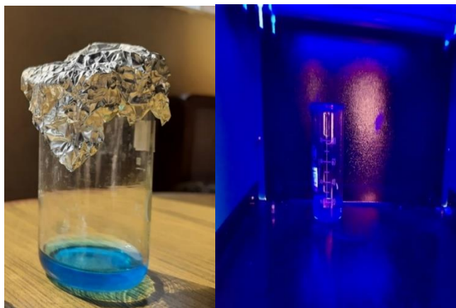
Figure 4 Photocatalytic degradation of MB under sunlight and under UV at 365nm
