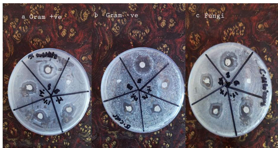
Figure 21 Zone of inhibition test for 1%CTAB-PAN fiber
