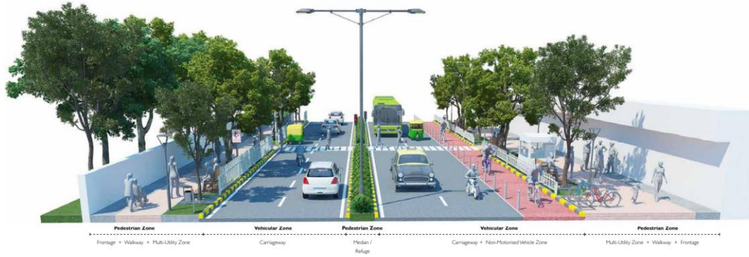
Figure 2-33 Complete Street Design Source: Street Design Guidelines
