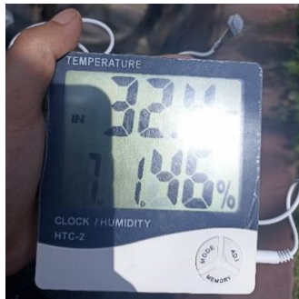
Figure 5-1 Digital Thermo-hygrometer HTC -2
