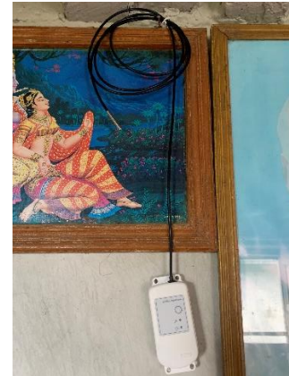
Figure 62 Data logger inside the traditional building
