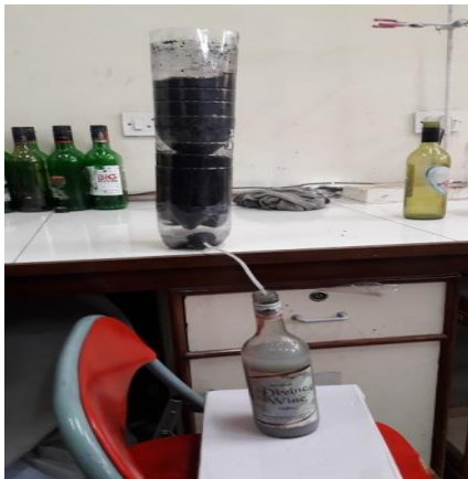
Figure 3.4 Filtration by using char
