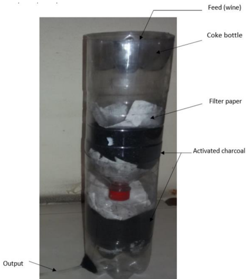
Figure 3.3 General setup prepared for charcoal clarification
