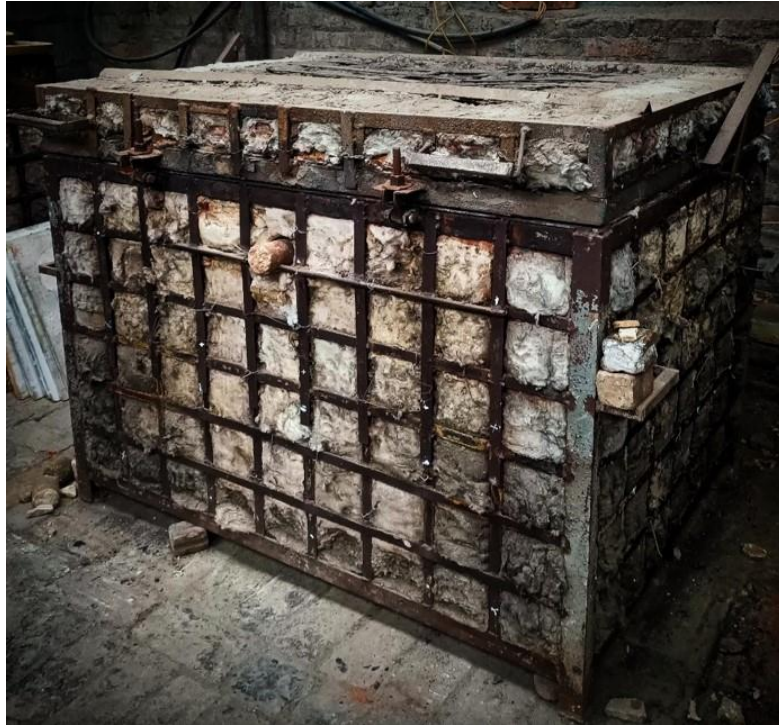
Figure: Electric resistance furnace at Everest Pottery
