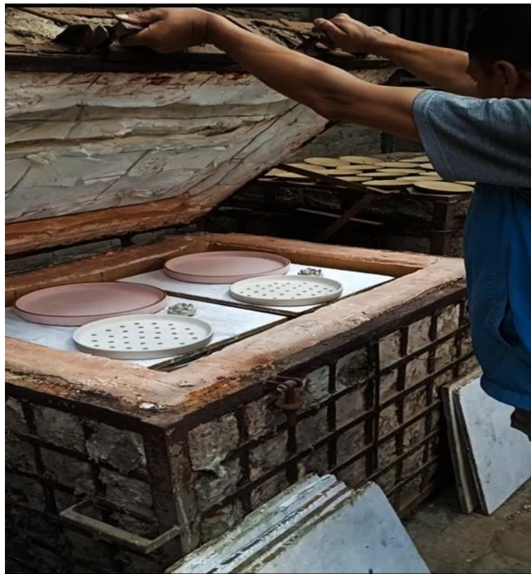
Figure: A fully loaded furnace ready for operation
