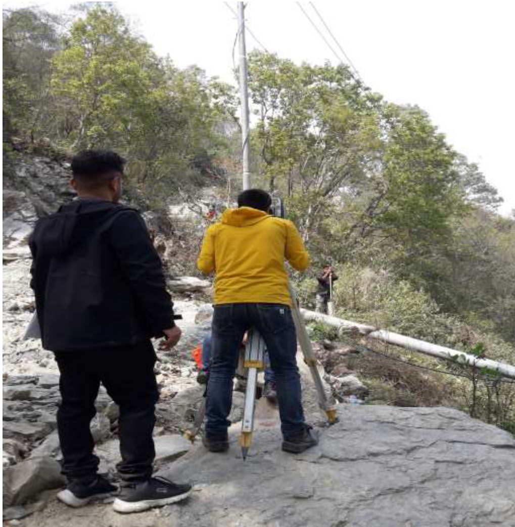
Figure 3. 4: Recording the data of Pillar number 7 using total station at the study area
