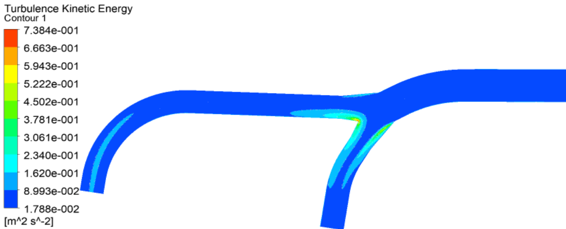
Figure D5: Turbulent Kinetic Energy Contour (Bend angle 28°)
