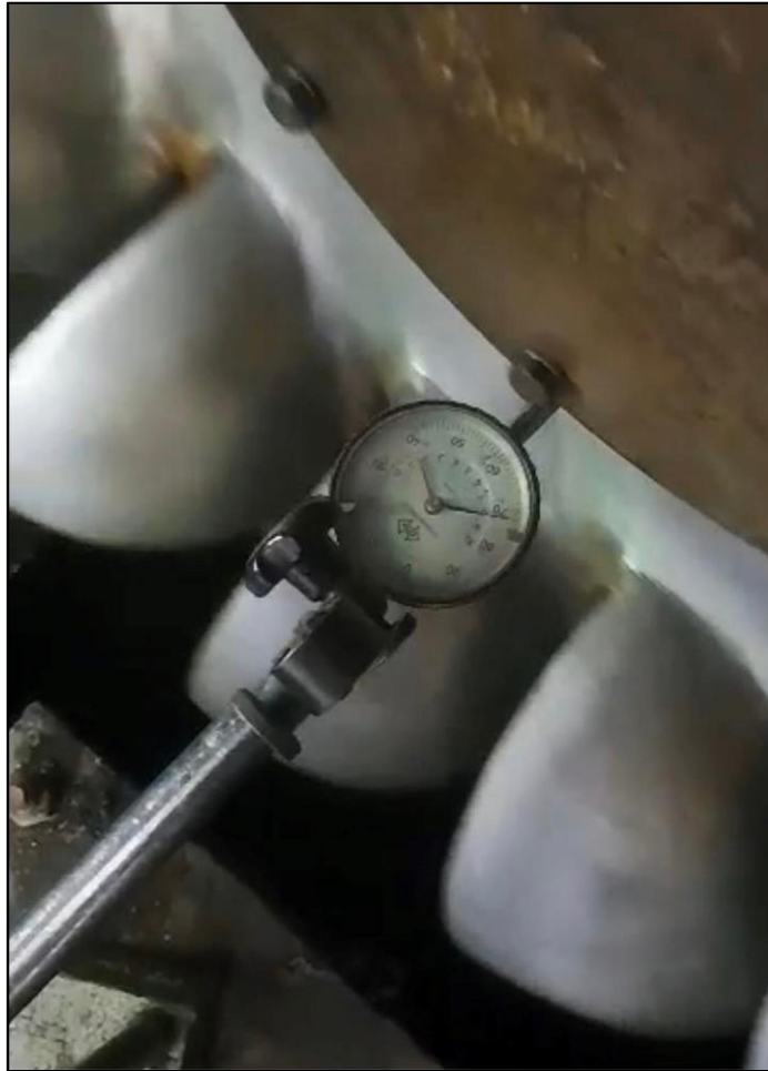
Figure 3.11: Eccentricity Measurement Using Dial Gauge
