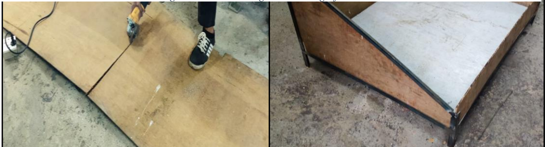
Figure 3.11: Outer cover made from plywood
