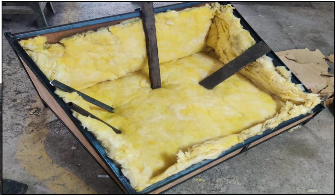
Figure 3.14: Glass wool as insulating material
