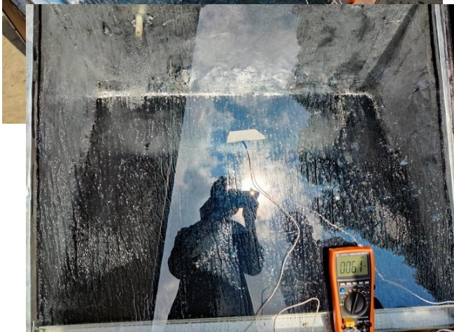
Distilled water collection during experiment from solar still
