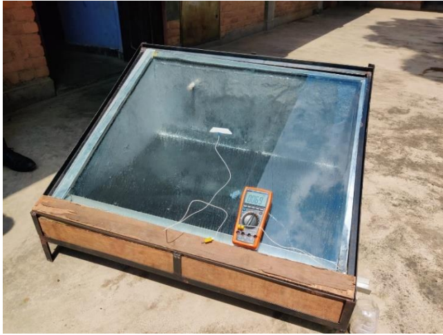
Evaporation process during experiment in solar still
