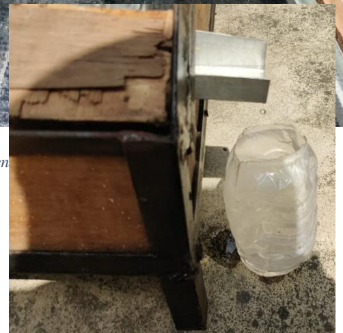
Distilled water collection during experiment from solar still
