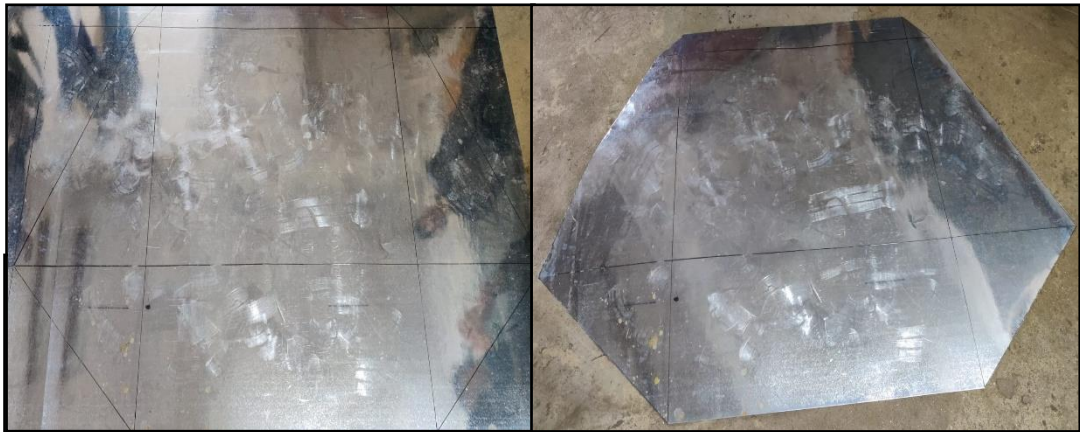
Figure 3.12: Marking and Cutting of GI Sheet
