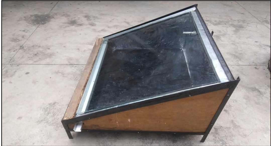
Figure 3.17: Fabricated solar still corresponding productivity was noted.
