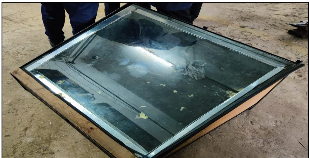
Figure 3.16: Placement of glass cover
