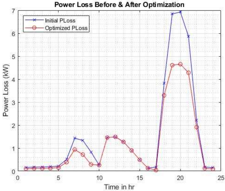
Figure 4. 8 Real power (kW) loss condition before & after optimization of the network for MPVCL
