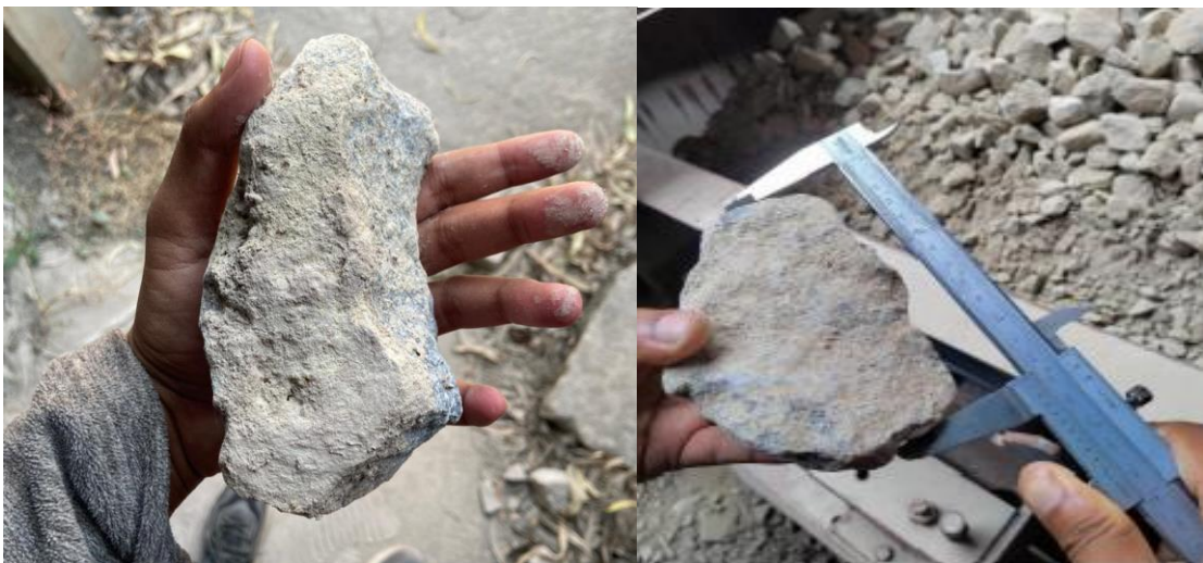
Figure 4-5: figure: Oversized crushed limestone from secondary crusher
