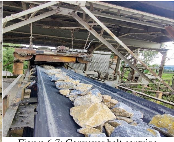
Figure 6-7: Conveyor belt carrying limestone to SC
