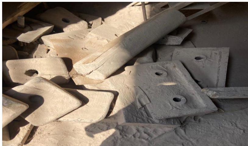
Figure 4-7: Worn out liner
