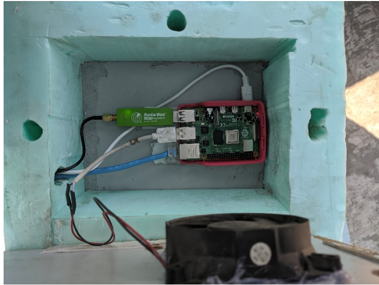
Figure 1: Physical Setup of ADS-B Ground Station
