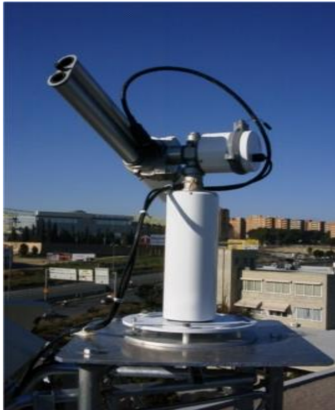
Figure 4: CIMEL Sun Photometer Deployed in AERONET Stations (Gregory, 2011).
