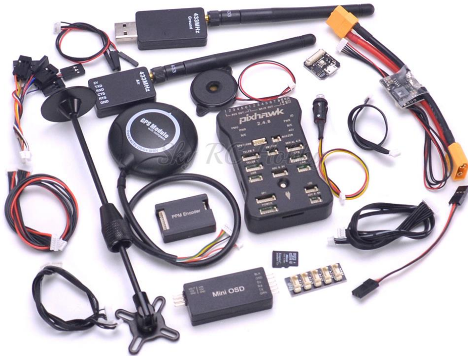
Figure 1.2: Pixhawk and its components (Source: alitools.com)
