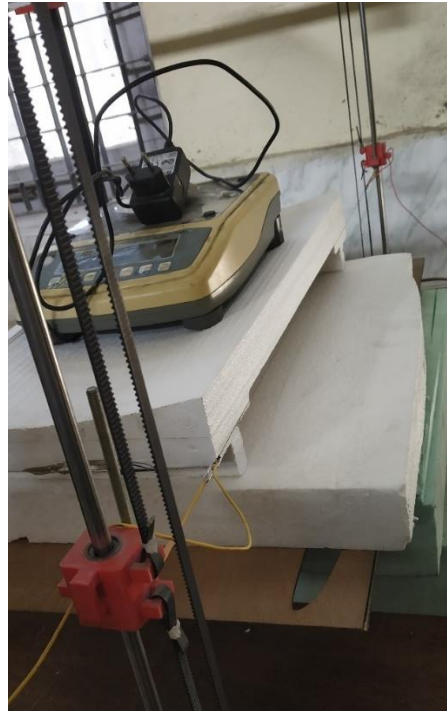
Figure 4.35: Cutting airfoil shape in CNC hot wire cutter
