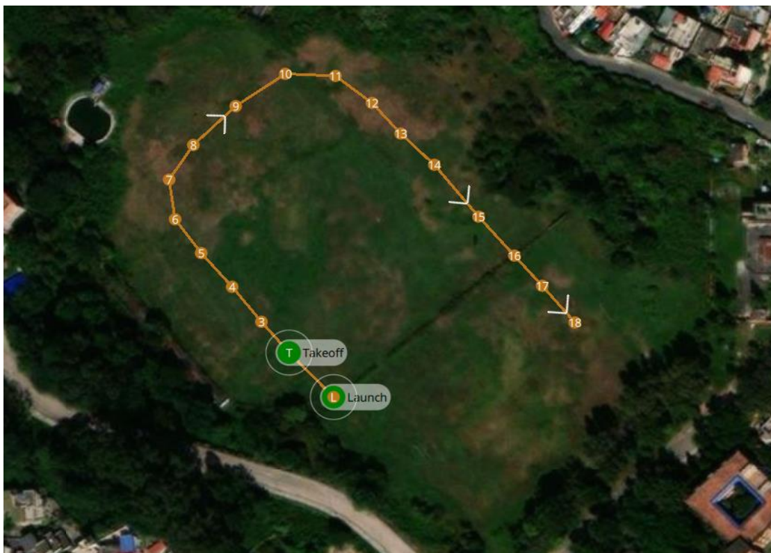
Figure 4.39: Initial flight plan for UAS in QGroundControl interface
