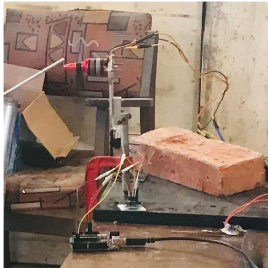
Figure 4.3: Thrust measurement of the selected motor
