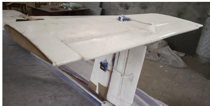
Figure 4.36: Empennage assembled with servo attached
