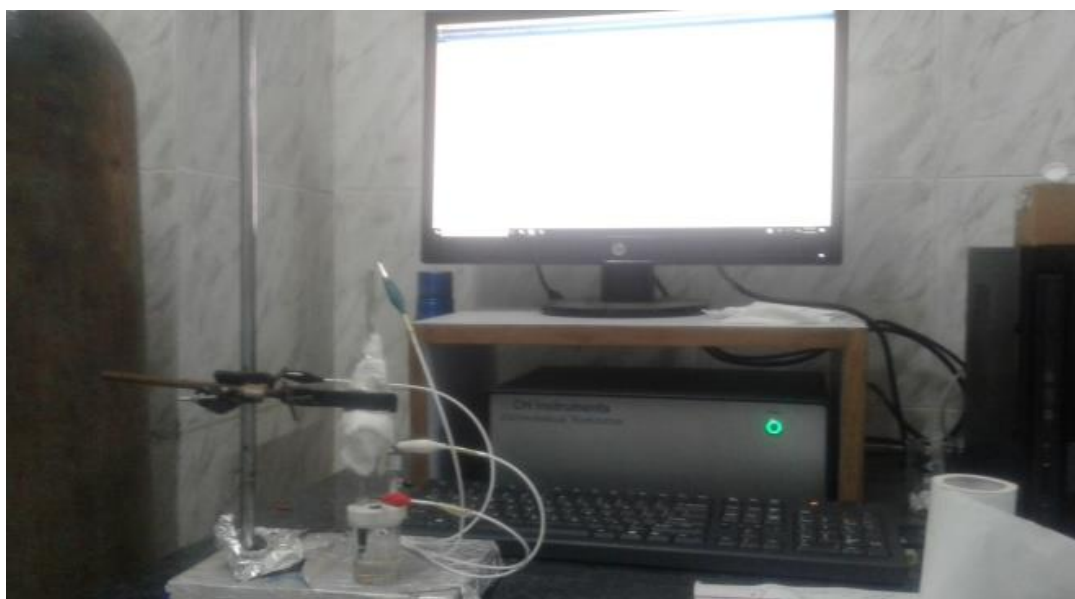
Figure 3. 13: Apparatus set up for electrochemical impedance spectroscopy using CH electrochemical workstation
