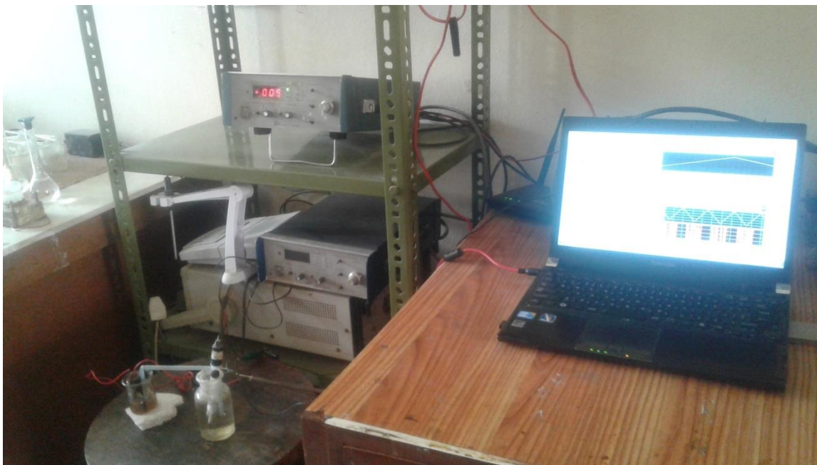
Figure 3.4: Apparatus set up for anodic polarization using Hokuto Denko HA-151 potentiostat
