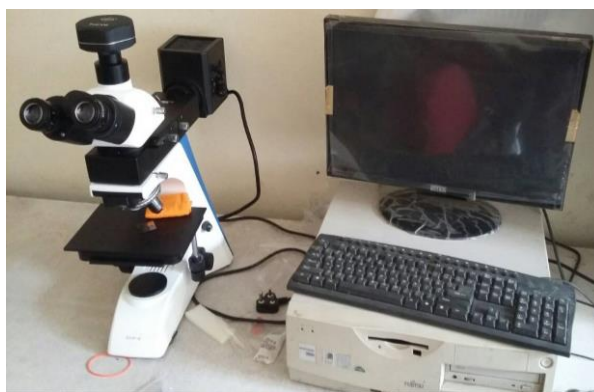
Figure 3.11: Optical microscope, Radical Scientific, India, reflection mode with an attached USB ProCam
