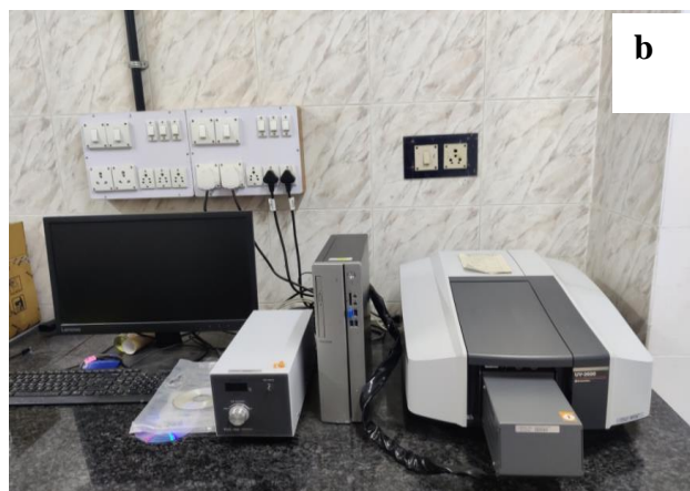
Figure 3.6: a. A schematic illustration of electron transition b. Shimadzu UV/Vis spectrophotometer
