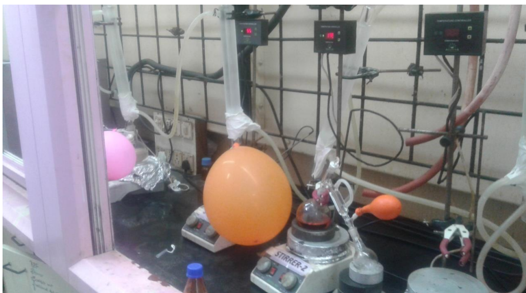
Figure 3. 1: Apparatus set up for distillation of aniline
