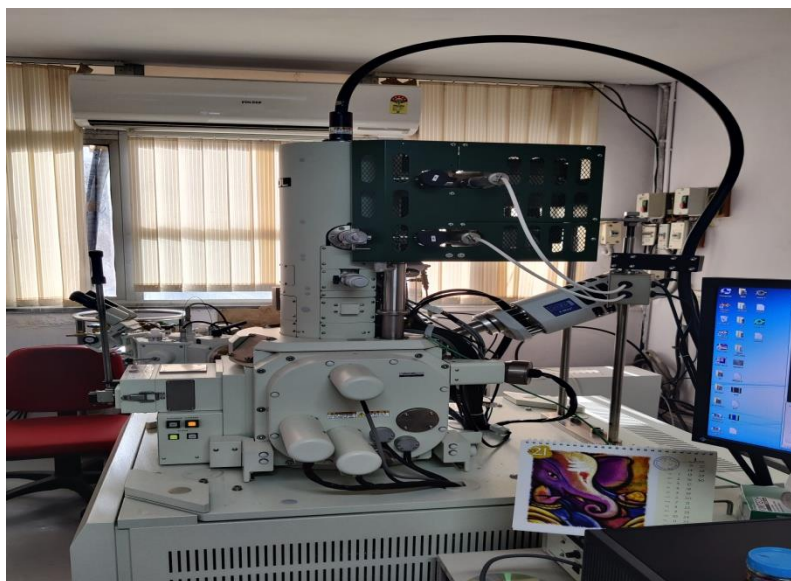
Figure 3.7: JEM-1200EX Scanning electron microscope in combination with an energy dispersion spectrometer (SEM-EDS)
