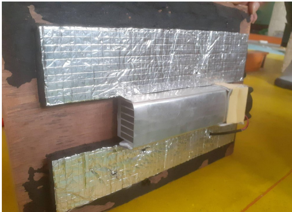
Figure: Tunnel Circulation of cold side air
