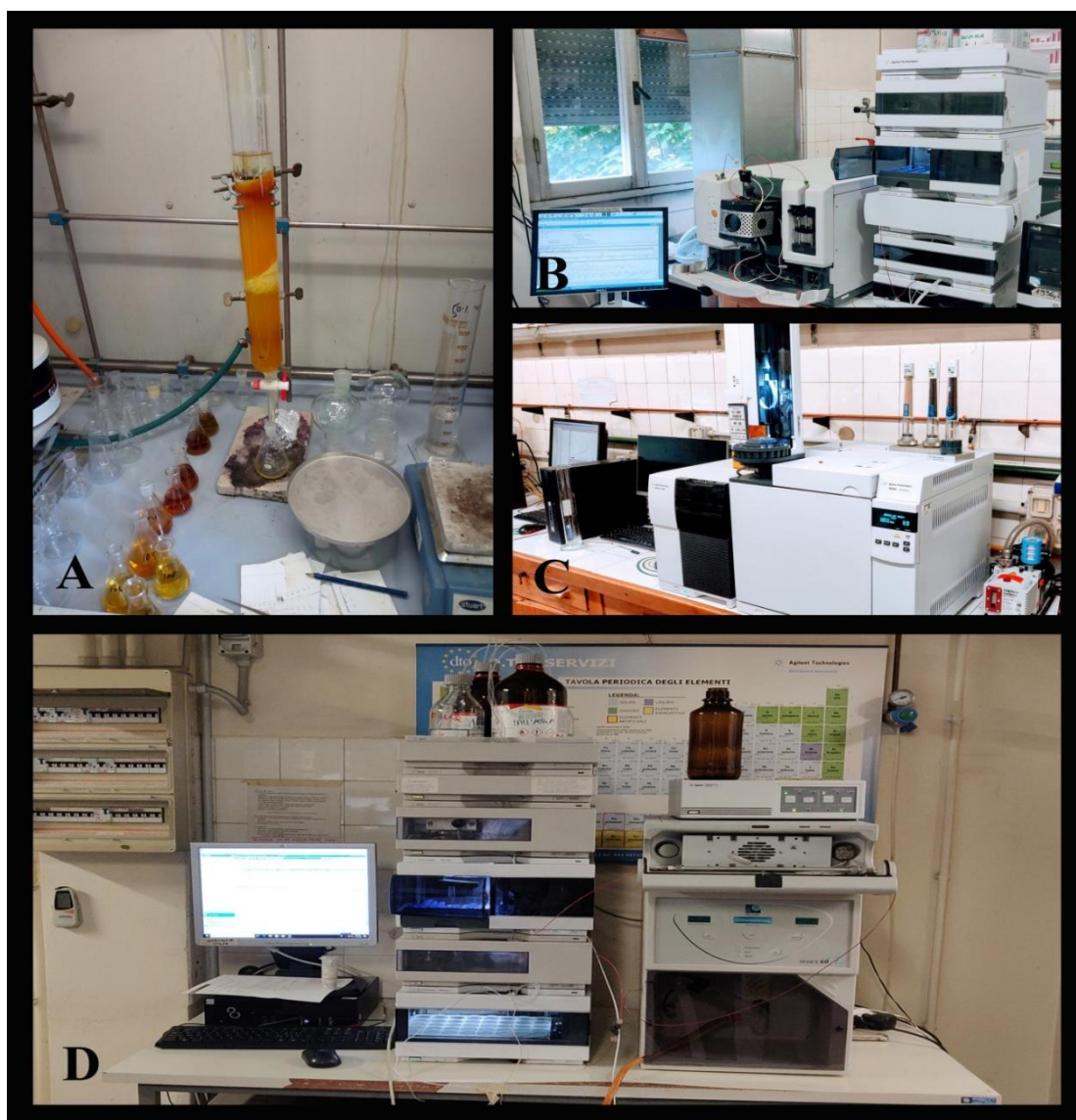
Photo plate 4: A. Chromatographic process; B. Liquid Chromatography (LC)-MS; C. Gas Chromatography (GC)-MS; D. High Performance Liquid Chromatography (HPLC)
