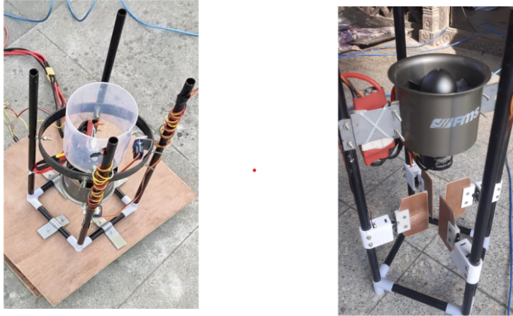
Figure 4.4: Contrasting Thrust Vectoring Mechanism (TVC). First image is the use of nozzle while second is of use of vanes for TVC
