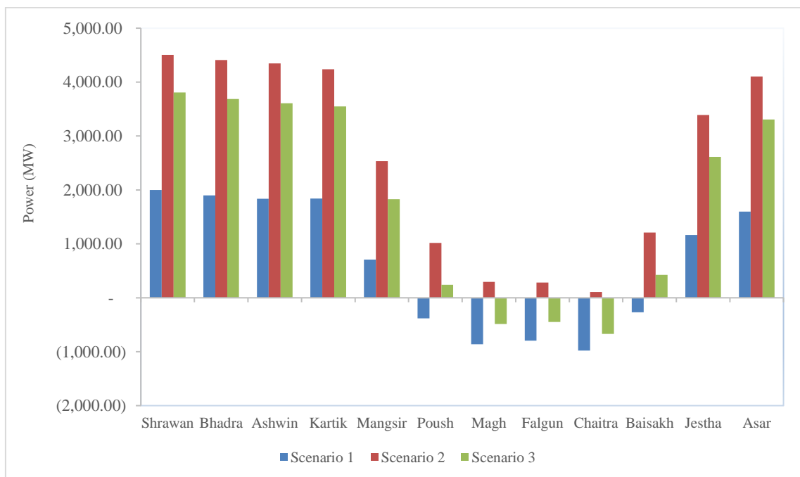
Figure 4-4 Capacity surplus/deficit during F/Y 2087/088 for different scenario
