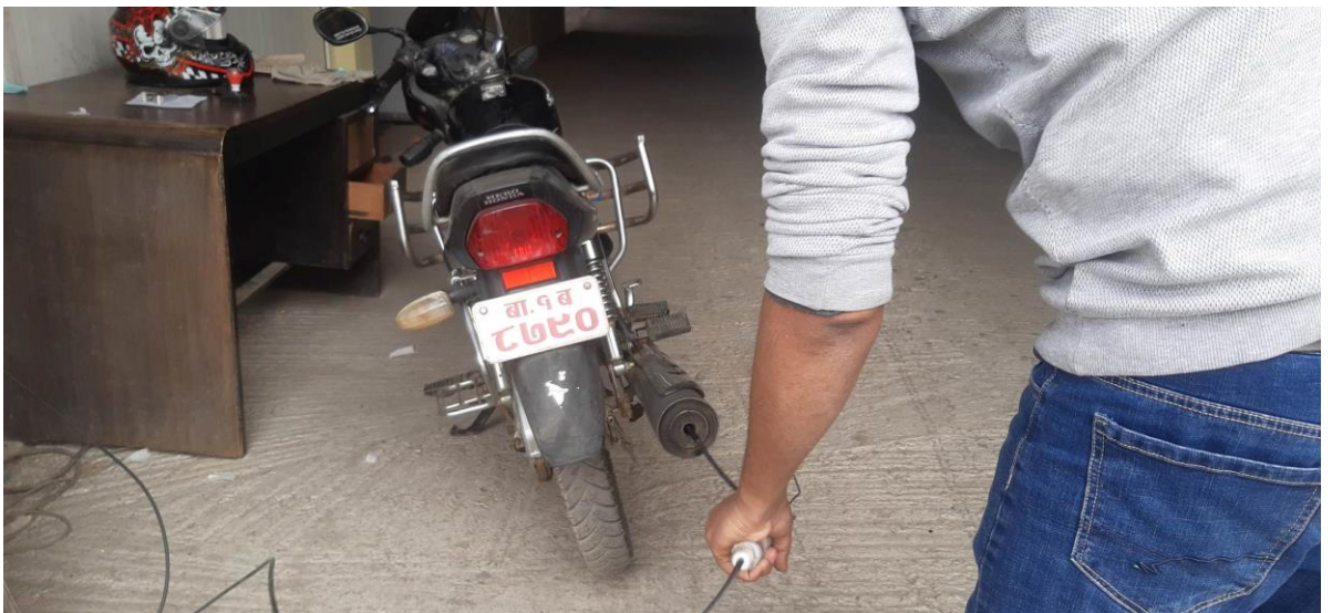
Figure 25: Emission test using flue gas analyzer
