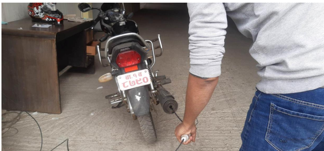
Figure 21: Emission being measured in Vehicle Fitness Test Centre (VFTC), Teku
