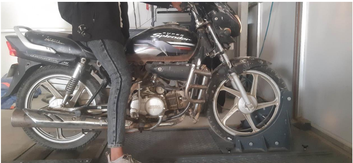
Figure 10: Chassis dynamometer test performed in Vehicle Fitness Test Centre (VFTC), Teku
