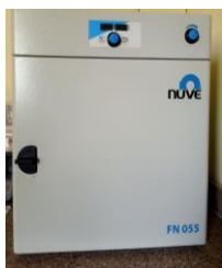
High precision Hydrothermal Oven (20-300 °C, \pm 2^{\circ}\text{C} ) Equipment
