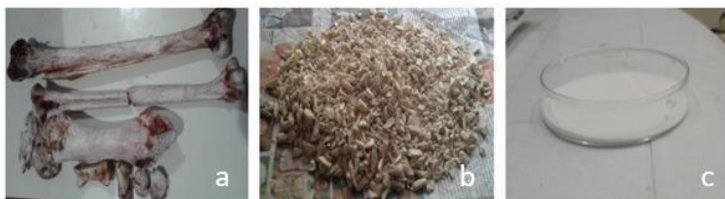
Figure 26: Photographs of (a) raw bones, (b) its pieces and (c) bone powder after grinding
