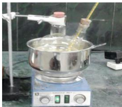
Figure 27: Photograph of alkaline hydrothermal hydrolysis to remove impurities from bone powder
