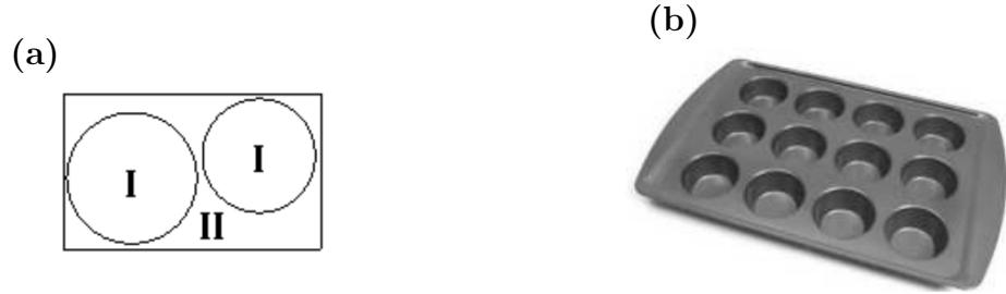
Figure 4: (a) Partition of the unit cell into atomic spheres (I) and an interstitial region (II), (b) Mufin-tin potential model (Pashov et al. , 2020).
