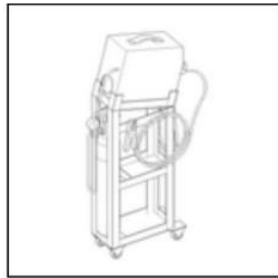
MIG WELDERS Metal inert gas welding: a welding process where the filler metal wire supplies the electric current, which is shielded from the access of air by an inert gas.
