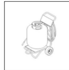
SAND BLASTER A blast of air or steam carrying sand at high velocity to clean metal surfaces.
