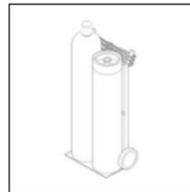
OXY-ACETYLENE RIG A welding process in which coalescence is produced by a flame of oxygen and acetylene gases mixed together at the point of ignition.
