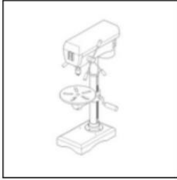
DRILL PRESS A machine used to drill or enlarge a cylindrical hole in a workpiece or part.
