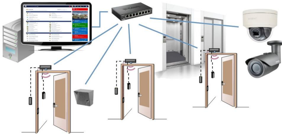
Figure 7-18 Access Control System
