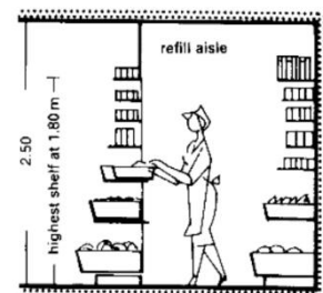
2 Partition allowing replacement of containers from refilling aisle
