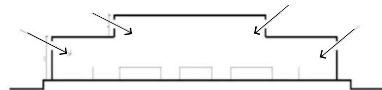
Figure 3-6 Natural light penetration from roof
