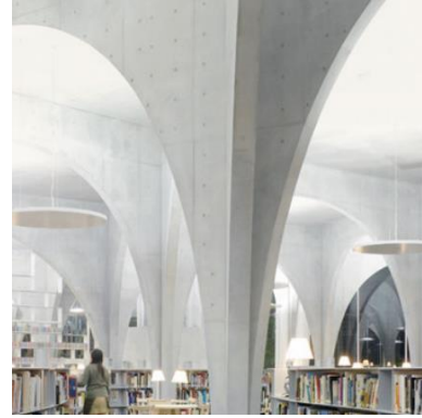
Figure 46: Tama Art University Library, Tokyo, Toyo Ito, 2007. Suspended fixtures with upward-pointing light sources provide an even luminous ceiling plane and a glare free base illumination for the stack and reading space.
