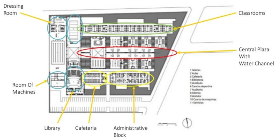
Figure 28: Zoning and Master Plan of Center for the Blind and Visually Impaired
