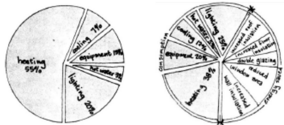
FIGURE 101 I) TYPICAL ANNUAL ENERGY CONSUMPTION AND II) POSSIBLE SAVINGS IN ANNUAL ENERGY CONSUMPTION (SOURCE: US ARMY)
