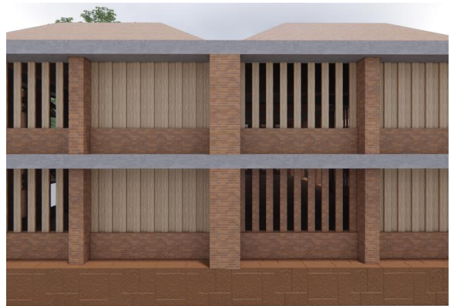
Figure 103 Detail of battens converted to sliding window and rendered view
