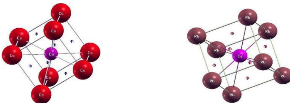
Fig. 1: (a) Unit cell of \text{CsCaH}_3 and (b) Unit cell of \text{RbCaH}_3 .
