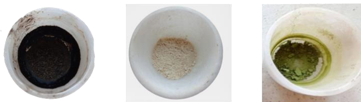
Fig 10: Powder of copper oxide, zinc oxide and copper-zinc nanoflakes
